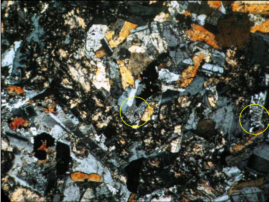
Figure 10. Photomicrograph of dolerite (X 4 magnification) under plane polarised light. This dolerite is composed of crystals of plagioclase, clinopyroxene and mignette. Intergrowths of quartz and alkali-feldspar (granophyric texture) are common (yellow rings).
